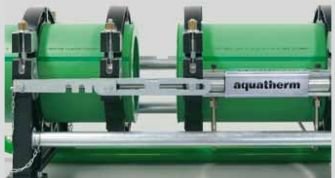
Divide the machine slide, remove heating element
