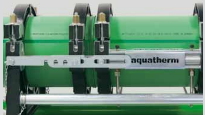
Join the pipes, cool down under pressure
