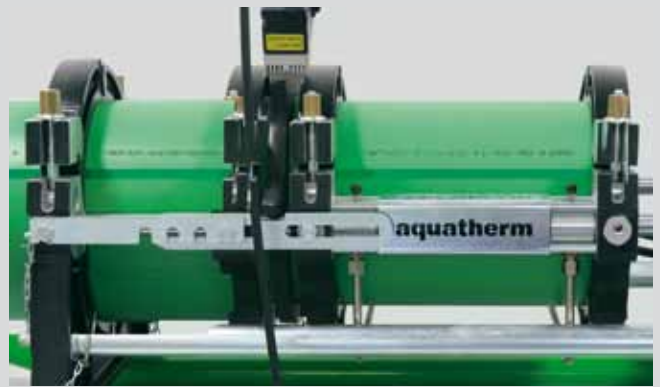
Positioning of heating element
