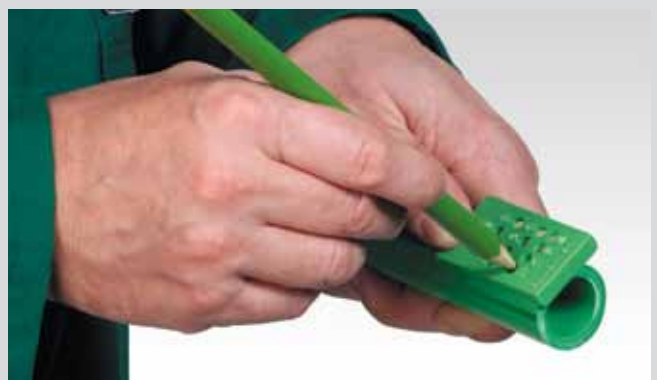
Marking of the welding depth
