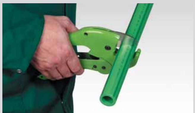
Cutting of the pipe
