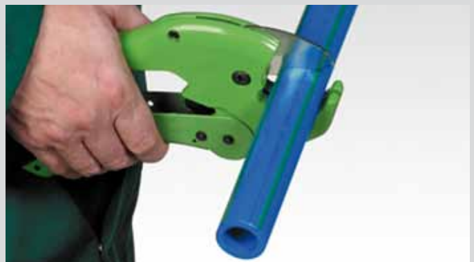
Cutting of the pipe
